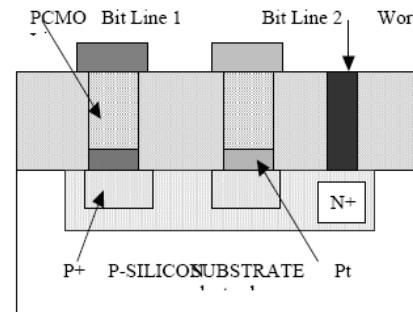
Fig.3 Resistor/diode memory array cell structure. Both top and bottom electrode of the memory resistor is made of Pt. The cell size can be as small as  $4\text{F}^2$ . This memory array required positive pulse for bot write and reset programming
