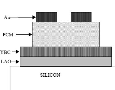
Fig.1 Pulsed Laser Deposited (PLD) test memory resistor structure. The memory material is PCMO ( $\text{Pr}_{0.7}\text{Ca}_{0.3}\text{MnO}_3$ ). The double bottom electrode is formed with YBCO ( $\text{YBa}_2\text{Cu}_3\text{O}_{7-\delta}$ ) on LAO ( $\text{LaAlO}_3$ )
