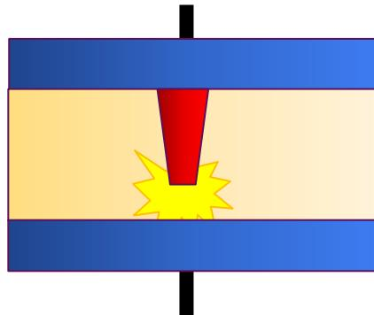
Absence of oxide thickness effect on  $V_{SET/RESET}$  indicative of LOCAL filament switching
