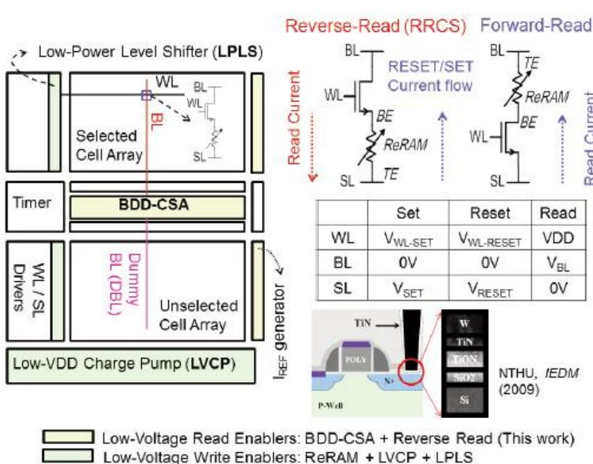
Figure 25.7.1: Block diagram and cell structure of the low-voltage ReRAM macro.
