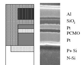
Fig.5 TEM microphotograph of a 1RID memory cell. Shallow P+ layer is formed onto n bit line. The memory array interconnect is copper doped Al.
