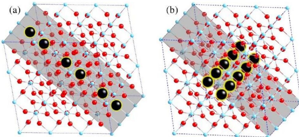
Fig. 1. Schematic picture of the oxygen vacancy chain system in  $3 \times 3 \times 4$  supercell of rutile  $\text{TiO}_2$ . The red represents oxygen, the blue represents Ti, and the black represents the oxygen vacancy. All oxygen vacancies are on the same (110) plane. (a) [110] vacancy chain. (b) [001] vacancy chain.
