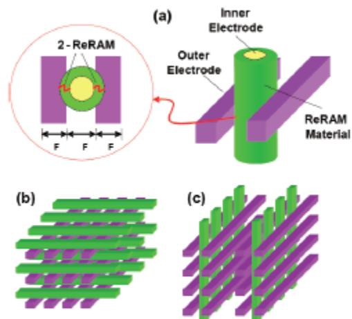
Fig. 1 Schematic diagram of (a) an unit vertically-defined ReRAM cell, (b) horizontal cross-point architecture (HCPA), and (c) vertical cross-point architecture (VCPA).
