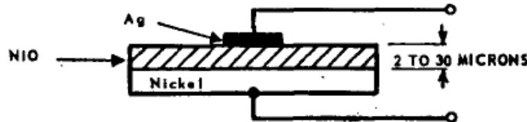
FIG. 1. Schematic representation of basic NiO thin-film device.
