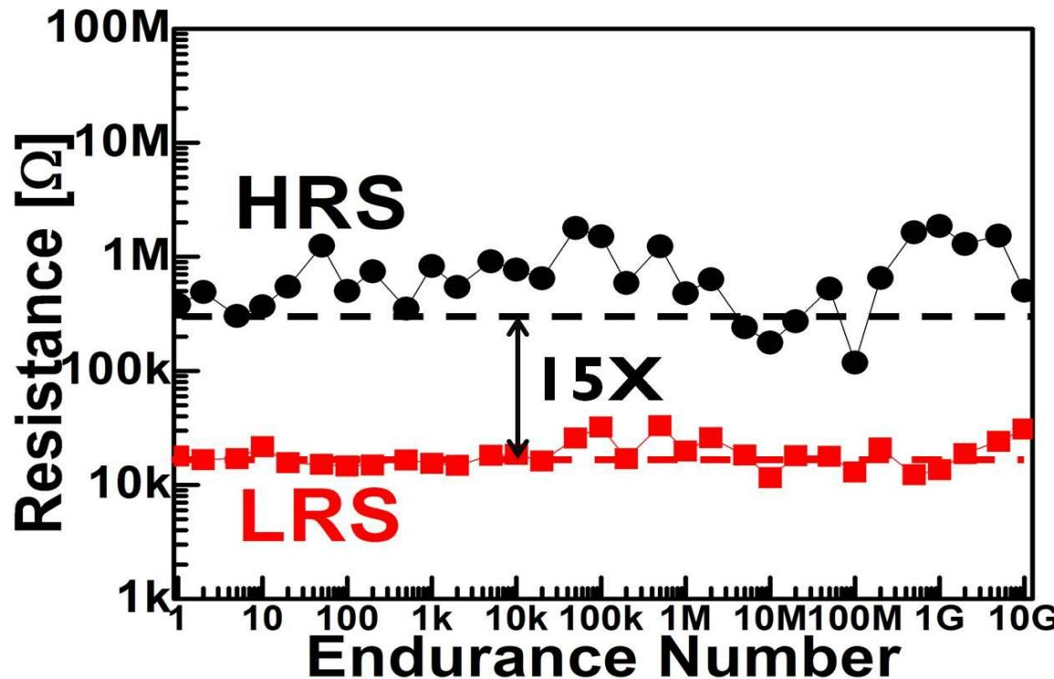
By balancing the SET pulse  $\text{WL}=1\text{V}$ ,  $\text{BL}=1.8\text{V}$ ,  $5\text{ns}$  and RESET pulse  $\text{WL}=3\text{V}$ ,  $\text{SL}=1.8\text{V}$ ,  $10\text{ns}$ ,  $10^{10}$  pulse endurance could be achieved on  $40\text{nm}$   $\text{Hf/HfO}_2$  ITIR devices.
