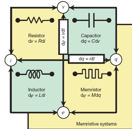
**Figure 1 | The four fundamental two-terminal circuit elements: resistor, capacitor, inductor and memristor.** Resistors and memristors are subsets of a more general class of dynamical devices, memristive systems. Note that  $R$ ,  $C$ ,  $L$  and  $M$  can be functions of the independent variable in their defining equations, yielding nonlinear elements. For example, a charge-controlled memristor is defined by a single-valued function  $M(q)$ .
