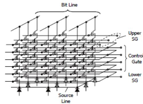
Fig. 4 Equivalent circuit of BiCS flash memory.
