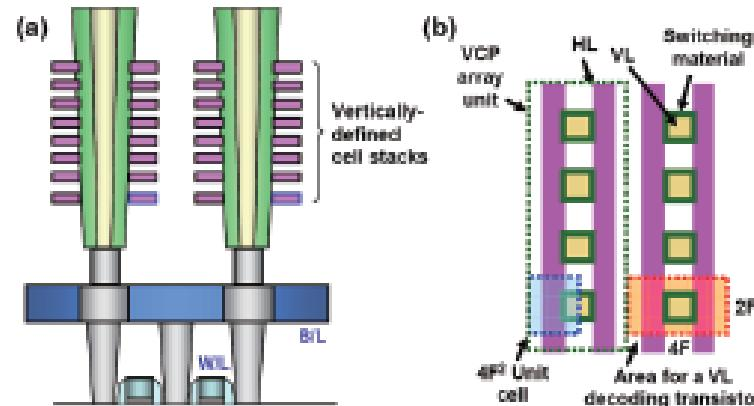
Fig. 10 (a) Vertical view and (b) top view of VCPA ReRAM with 4F<sup>2</sup> memory cell densities.
