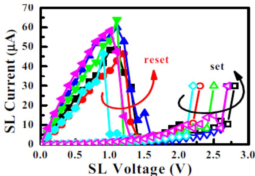
Figure 4 The DC-IV characteristics of two reproducible resistance states.
