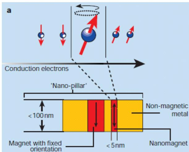
Magnetization of free layer in MTJ can be switched back and forth by switching current direction
