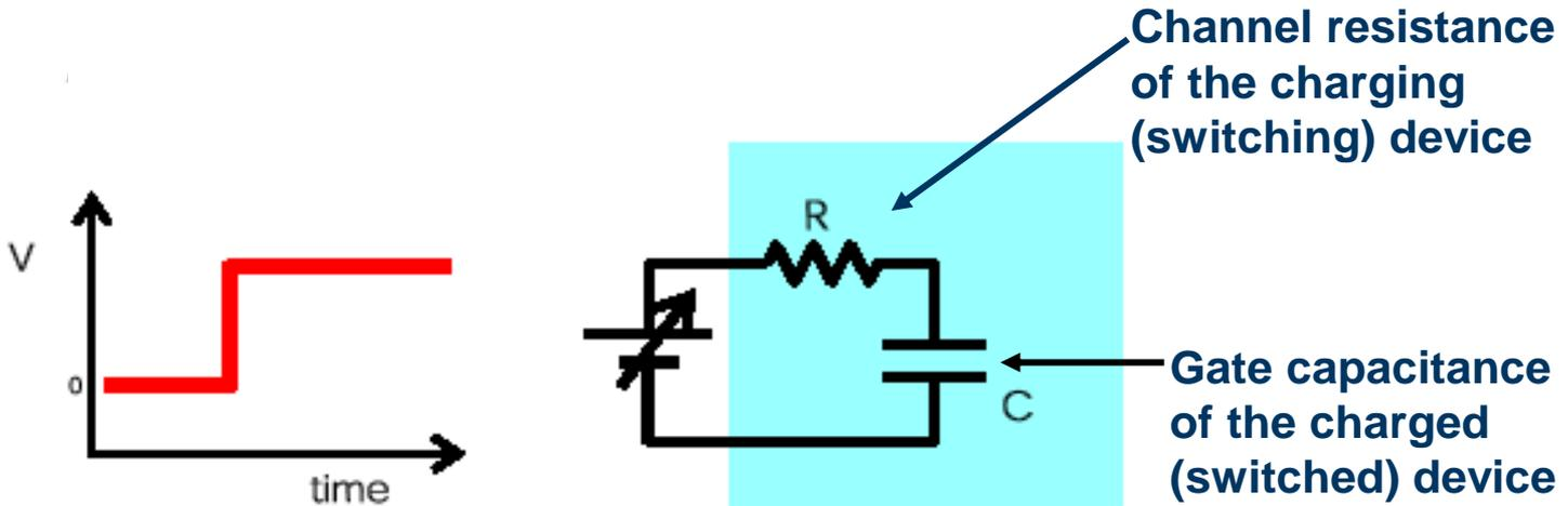
$$E_{\text{diss}} = \int_0^{\infty} i^2 R(t) dt = \frac{1}{2} CV^2 \quad (\text{independent of } R!)$$
