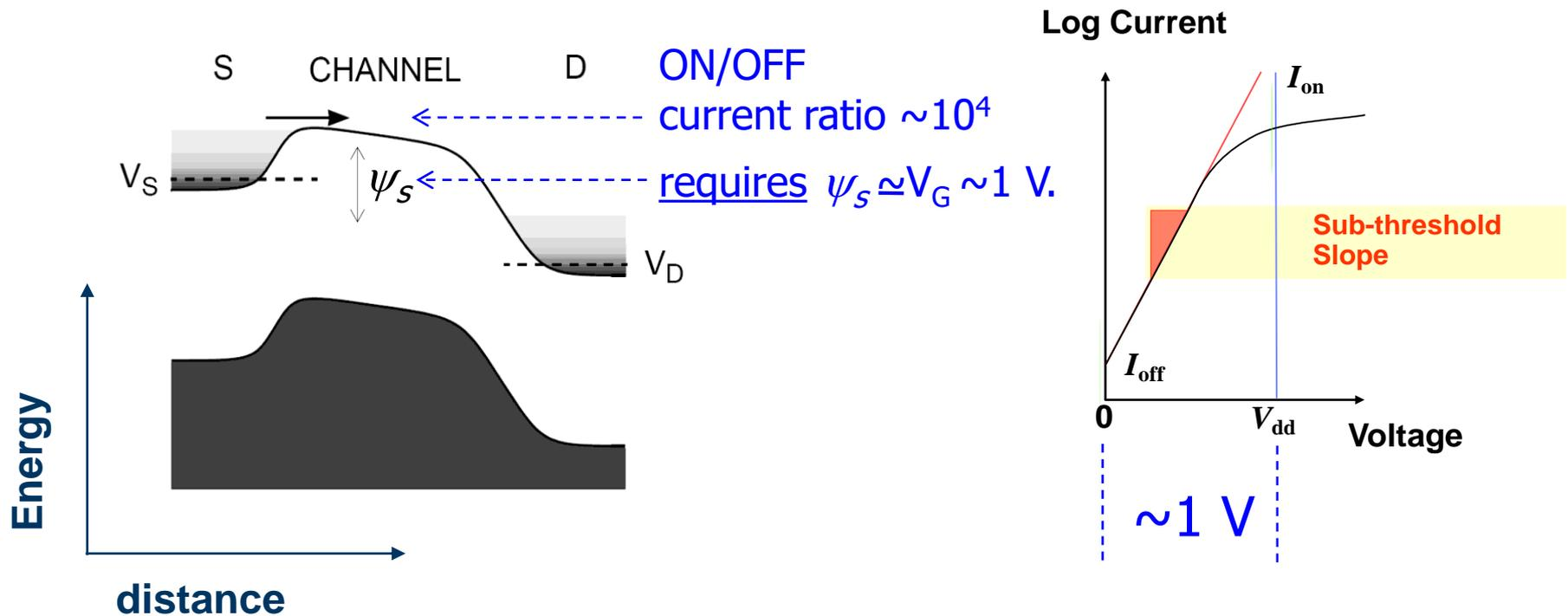
With voltage swing already reduced to  $\sim 1V$ , The FET is close to its fundamental voltage limit for operation at ambient temperatures.
